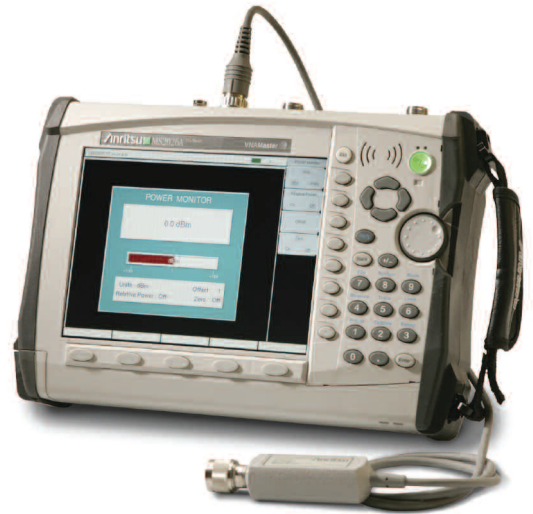
The easy-to-view Power Monitor display minimizes keystrokes when testing in the field.
